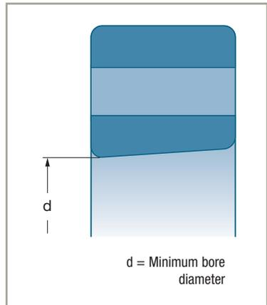
■ The 1:12 taper bore is produced in series on:
