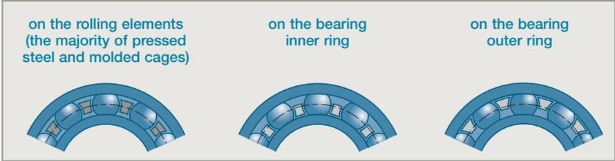
The centering choice depends on the bearing operating criteria: vibration, impacts, high speeds, speed variations,...
